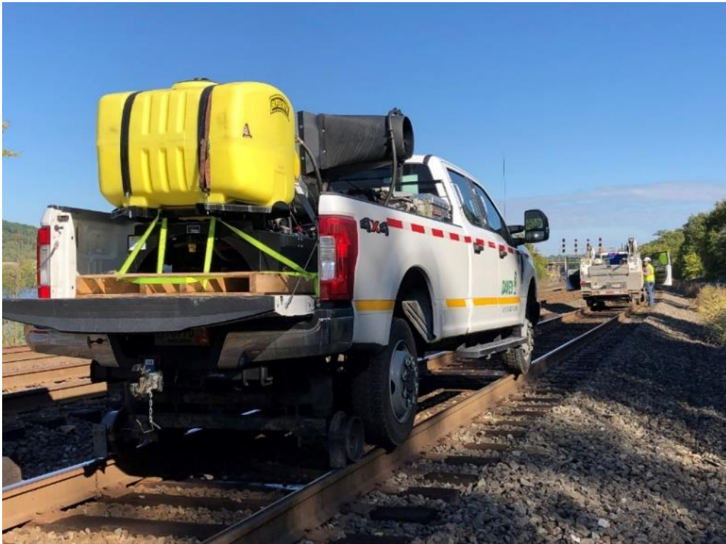
Figure 6. Mist blower that will be used on railways to treat SLF.
