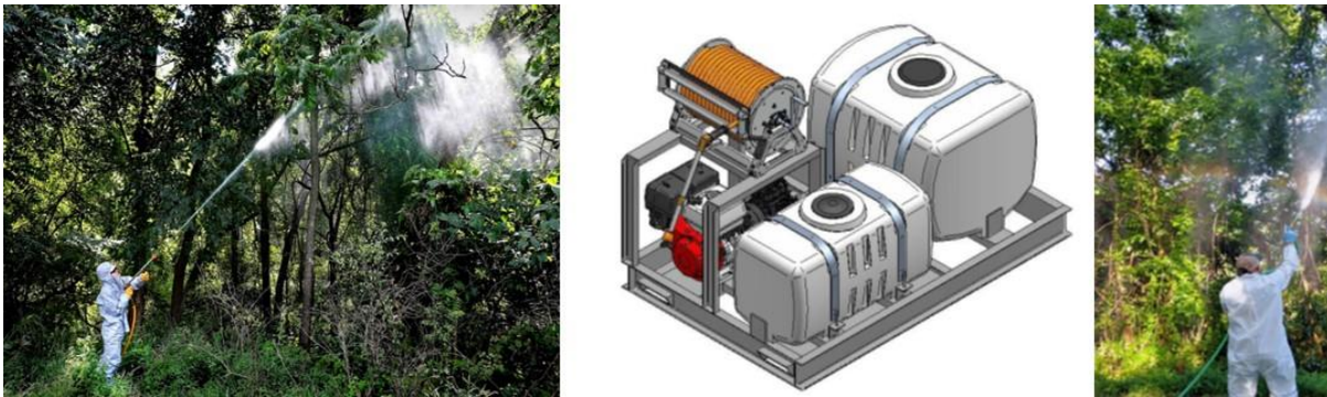
Figure 5. SLF insecticide treatments using pressurized equipment, and an example of spray tank and pump that is mounted onto a truck or ATV.
