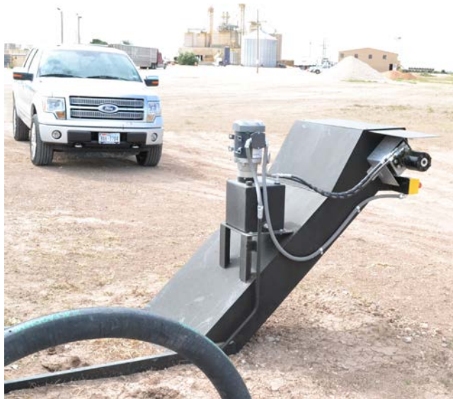
Figure 7. Waste discharge point. Material is discharged with 2% to 3% moisture content.
