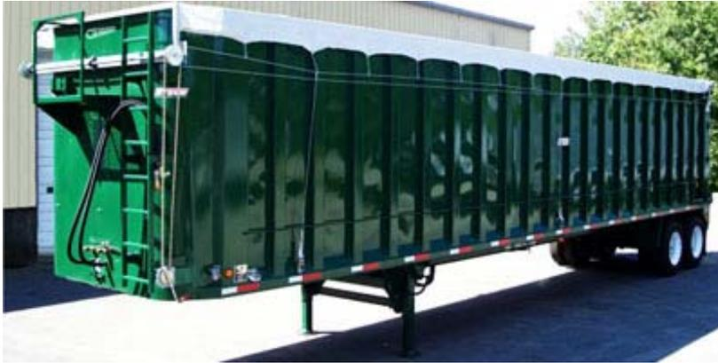
**Figure 4: Example of a tarp drawn tight over a trailer.**
