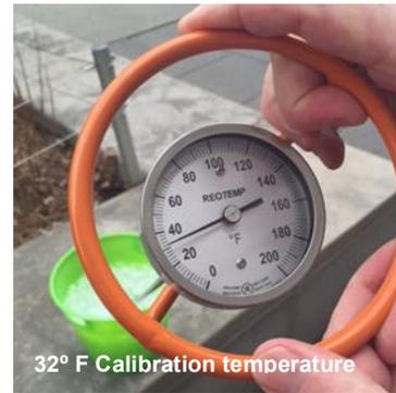
5. If the dial does not read 32°F, using the flathead screwdriver, turn the small (1/4") hex screw head on the back of the dial case of the thermometer until the pointer is at 32°F. Turn the screw counter-clockwise to increase temperature or clockwise to decrease temperature.
