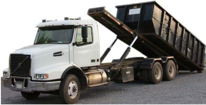
**Figure 5: Example of a roll-off truck trailer.**
