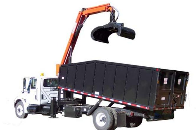
**Figure 2: Grapple truck with dump trailer.**
