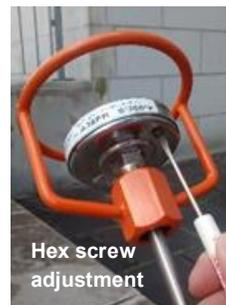
6. When adjustment is complete, re-check the thermometer in ice water. Repeat adjustment if necessary.
