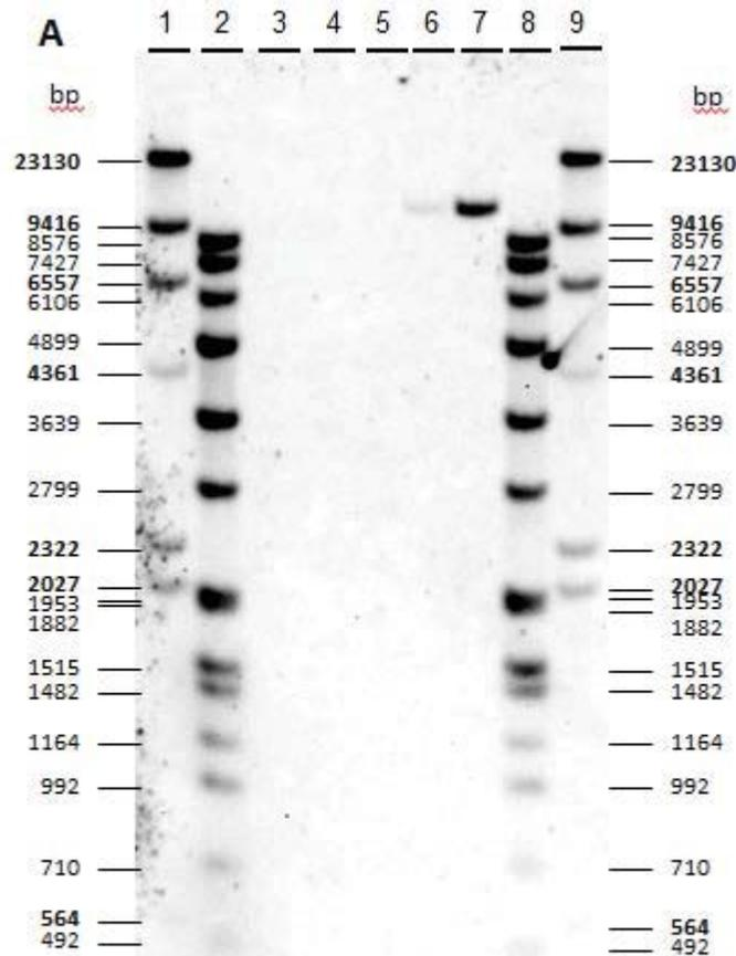
**Figure V-24: Hybridization performed with a vector backbone probe covering the 5'ORI pVS1 sequence (P025) to assess the vector backbone presence in the T<sub>2</sub> generation of MS11**
