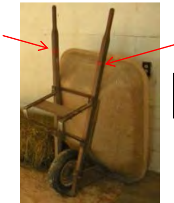
In the photograph, note the red tape on the handles; this is one way to designate area of use for equipment.
