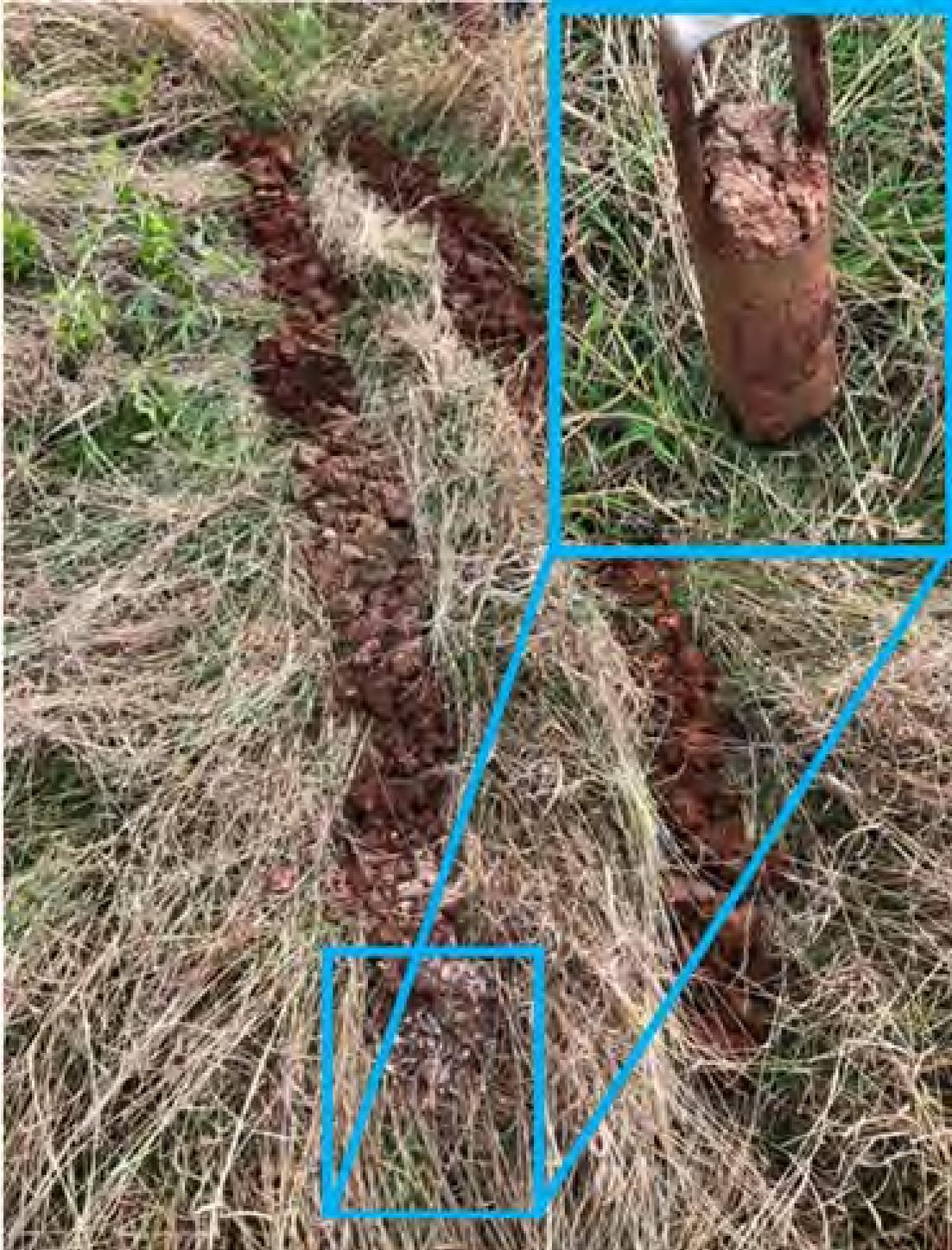
Figure 16. Photo of discolored, wet soil sample from Site 2
