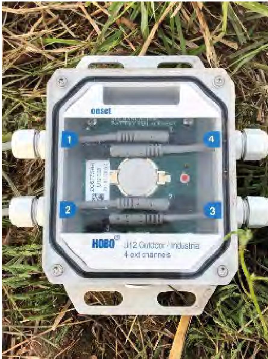
Figure 17. Onset HOBO U12 Data Logger
