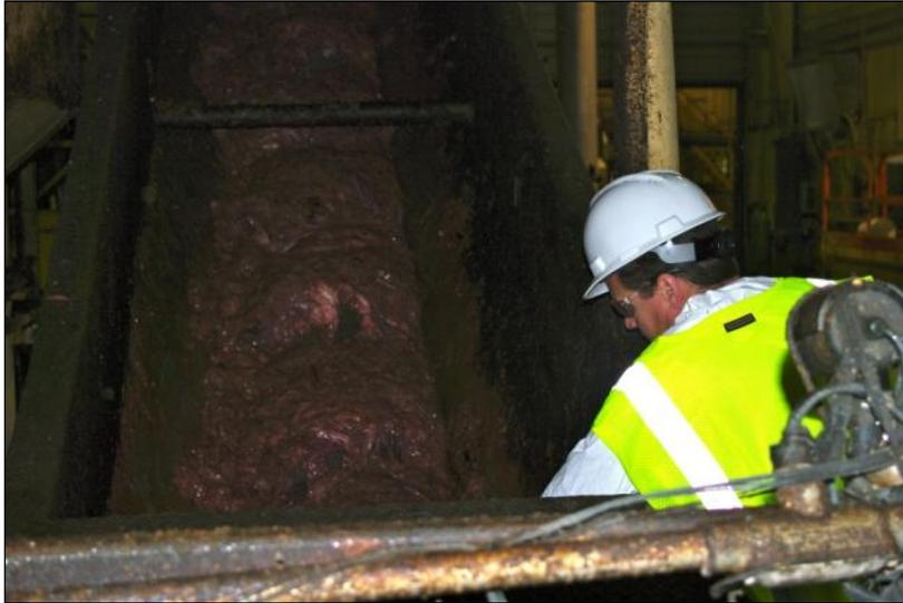
**Subject:** DATS wipe sampling wall of auger during processing of inoculated loads.
