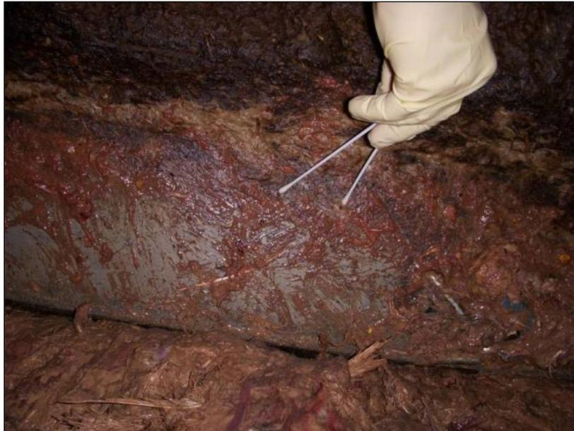
**Subject:** DATS collected samples 6a and 6b from the side wall of the incline auger.
