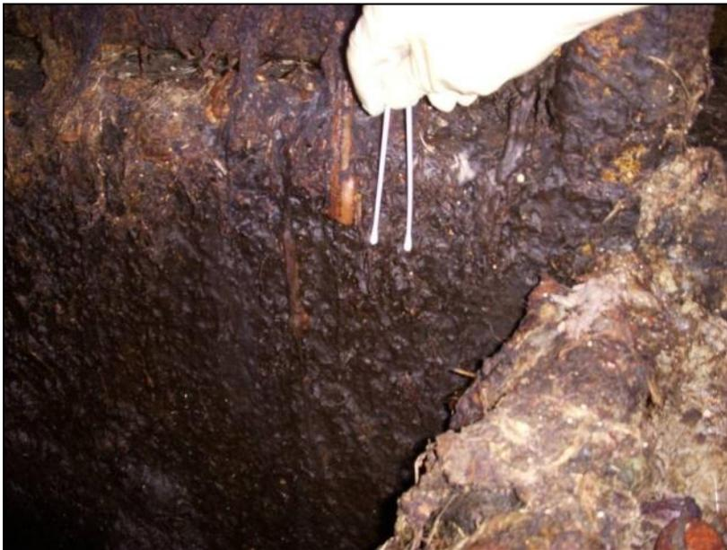
**Subject:** DATS collected swab amples 3a and 3b from the central vertical wall of the tipping floor pit.
