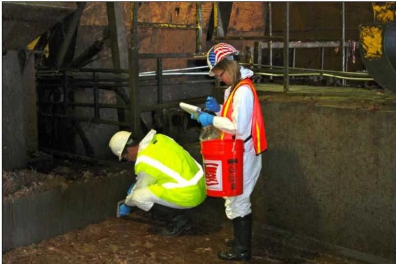
**Subject:** DATS collecting a sample from the wall of the tipping floor pit during the post-inoculation phase. Note that plant personnel frequently push material against this wall using a front loader and deposit it into the pit.
