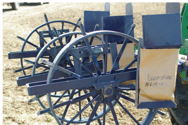
Mechanical wheel soil samplers like this one were used during the PCN survey in 2006.
