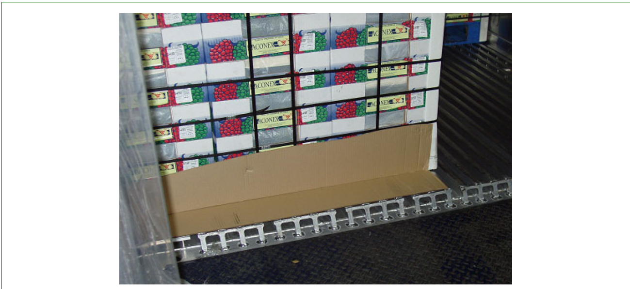
Figure 3-7-5 Proper Placement of Cardboard Between the Last Pallet Row of Fruit and the Back Doors of the Container
