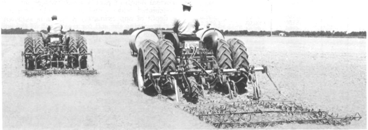
FIGURE 39.—Tractor applicators working in tandem. Scotch harrow pulled by each tractor seals the furrows opened by the shanks.
