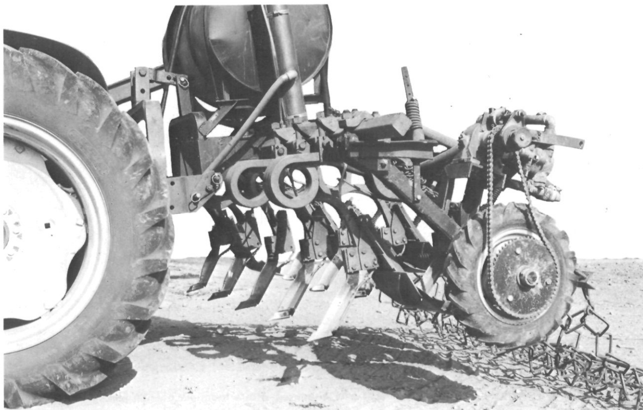
FIGURE 37.—Tractor applicator, showing shanks and ground wheel that operates variable displacement piston pumps. The wheel compensates for irregular speed of tractor and results in even discharge of chemical.
