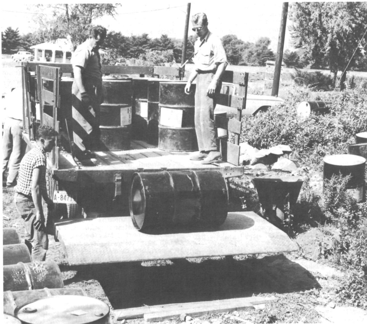
FIGURE 34.—Additional equipment, such as platform lift for moving drums of chemical, is useful. N-38184
