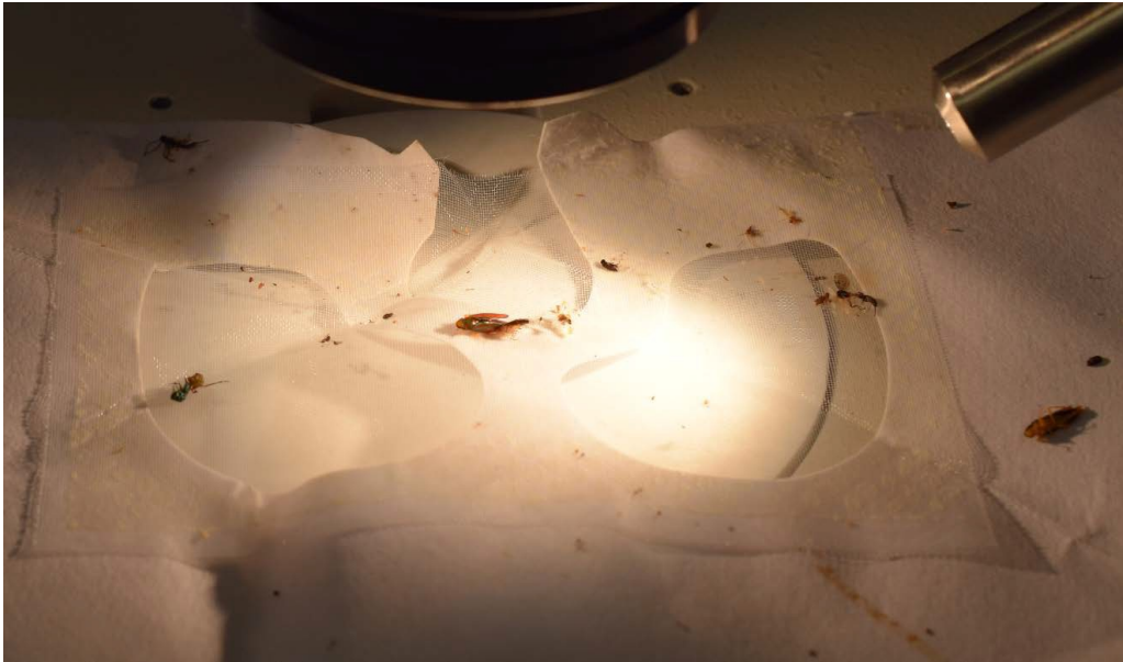
A filter paper spread out and ready for viewing under the microscope.
