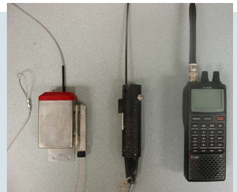
From left to right: a Telonics monitor, an ATS monitor, and an Icom receiver.
