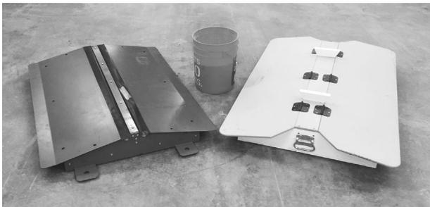
**Figure 2.** Prototype bait stations for invasive wild pigs designed to enable the evaluation of materials (metal or plastic) to construct a bait station that would maximize feeding by multiple individuals simultaneously in field trials with free-ranging wild pigs in September 2015, at Camp Bullis, San Antonio, Texas, USA.
