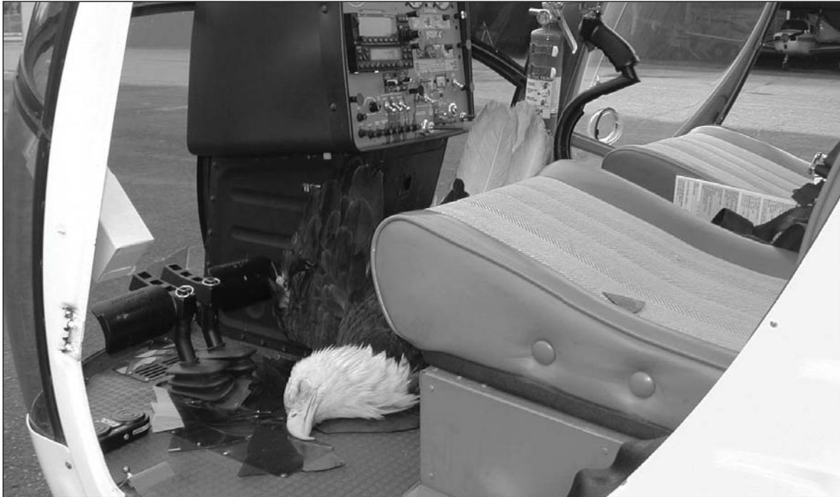
**Figure 2.** Damage to helicopter windcreens occur when wildlife, such as this bald eagle (*Haliaeetus leucocephalus*), collide with aircraft during flight. (Photo courtesy of Chris Cooper)
