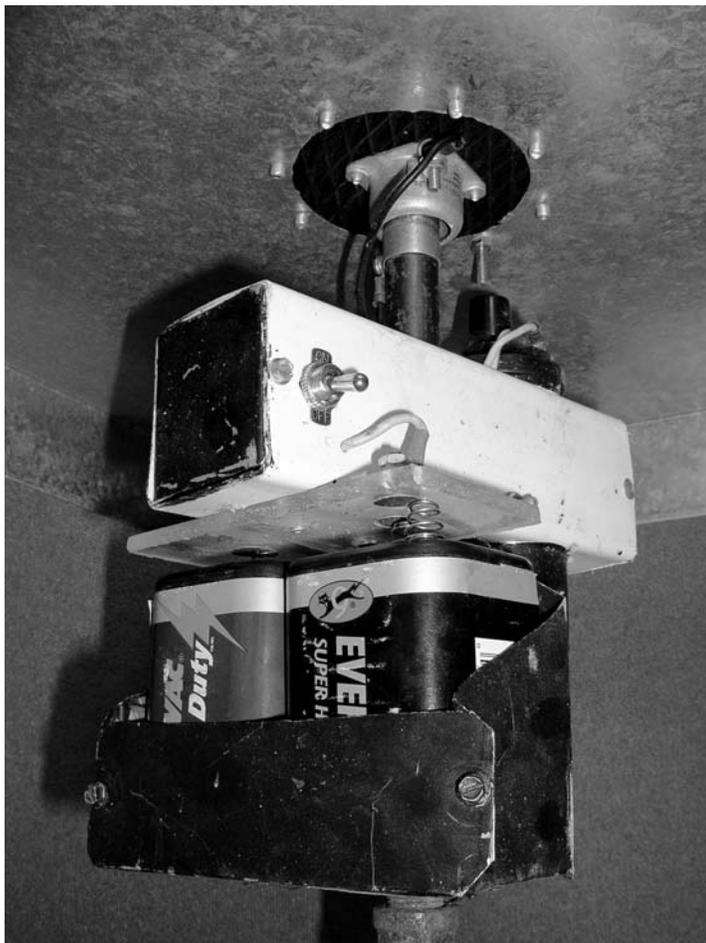
**Figure 1.** Underside of the Nuisance Bear Controller (NBC) showing the rubber matting attached to the trigger plate and wires running from the trigger plate to the vibrator coil/condenser. Two 6 volt batteries, linked in series, power the system but only when the trigger plate is moved up or down. Photo by N. Lance.
