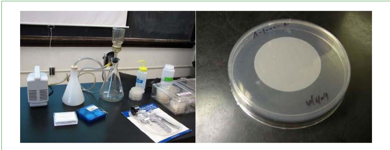
Figure 10-1-6 Vacuum Apparatus for Water Filtration and Filter Plated onto PARPH-V8 Plate 1
