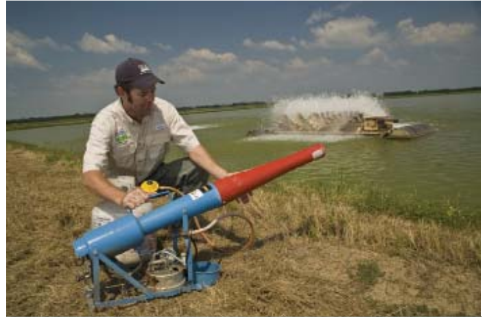
A propane cannon uses sound to scare birds and mammals from aquaculture operations, airports, and other locations where they can cause conflict.
