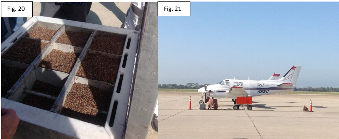
Fig. 20 - Aerial release box containing chilled sterile flies prior to their aerial release. Fig. 21 Beechcraft King Air contract aircraft used to disperse sterile insects over the Los Angeles Basin.
