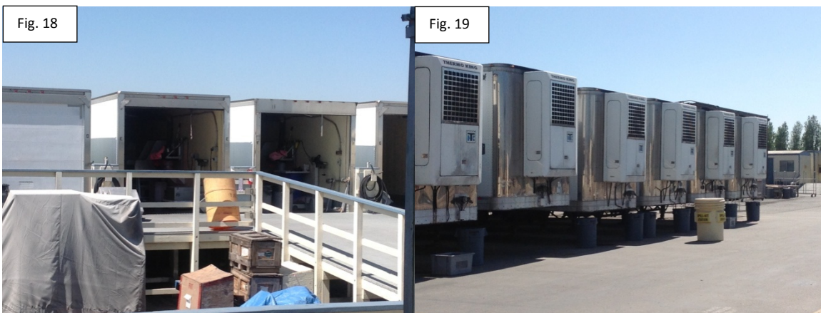
Fig. 18 & 19 - Front and back views of the refrigerated trailers used at Los Alamitos to chill sterile insects prior to their release. Thermo-King units operate on diesel. For reasons of fire safety, all trailers are grouped together.
