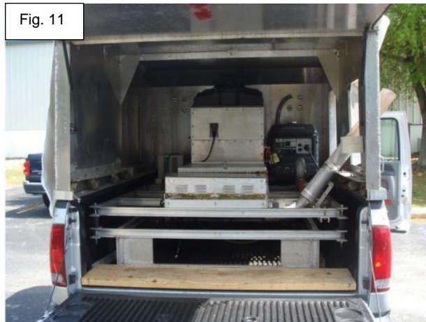
Fig. 11 - Chilled adult release machine with tube extending to the right side of the vehicle. DC converter and portable generator also are visible in photo.
