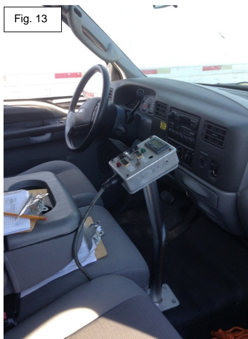
Fig. 13 - Controller for chilled adult release machine is mounted in truck cabin. The controller is used to set potentiometer (pot) settings affecting the rate of release.
