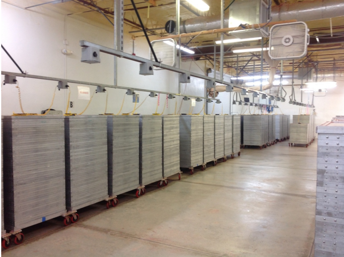
Fig. 5 - Large room at the Sarasota ERF shows placement of "towers" where sterile adult Med fly emerge and feed prior to release.
