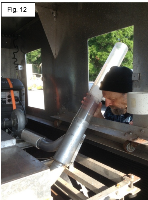
Fig. 12 - Earl Andress inspects side chute where chilled adults will be blown from moving vehicle away from traffic toward the shelter of trees and shrubs.
