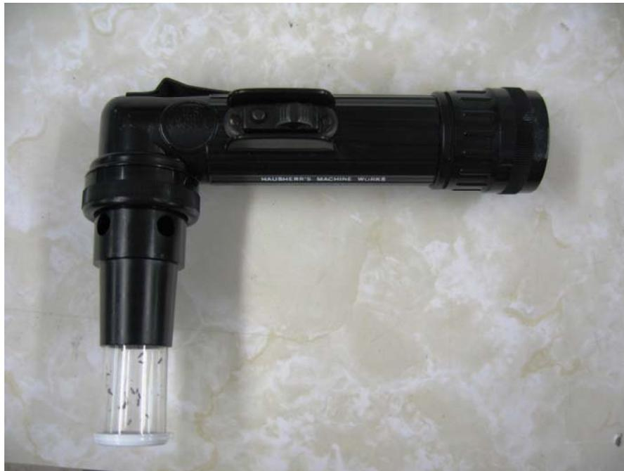
**Figure 1: Hand-held vacuum sampler for collecting psyllids**
