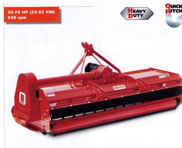
Figure 3. Example of a flail mower (Hurricane H70). Source: http://www.wikco.com/befh70.html (Accessed August 11, 2009.)
