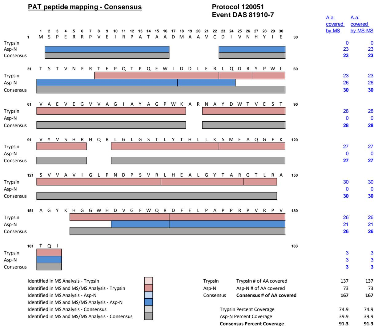
**Figure 64. Comprehensive MS and MS/MS Sequence Coverage Map for Trypsin and Asp-N digests of DAS-8191Ø-7 Cotton-Derived PAT**
