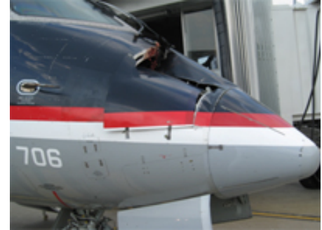
Damage caused by bird strike.
