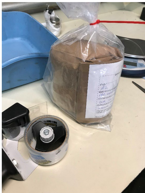
Figure 7. Final sample bag and Sample Information Form in plastic bag, sealed with a zip tie.
