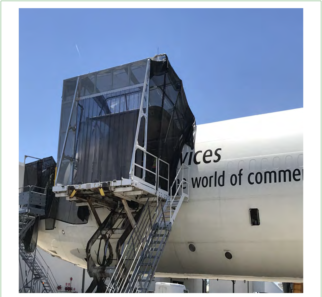
Figure 4-1 Example of a Cargo Exclusion Device 1
