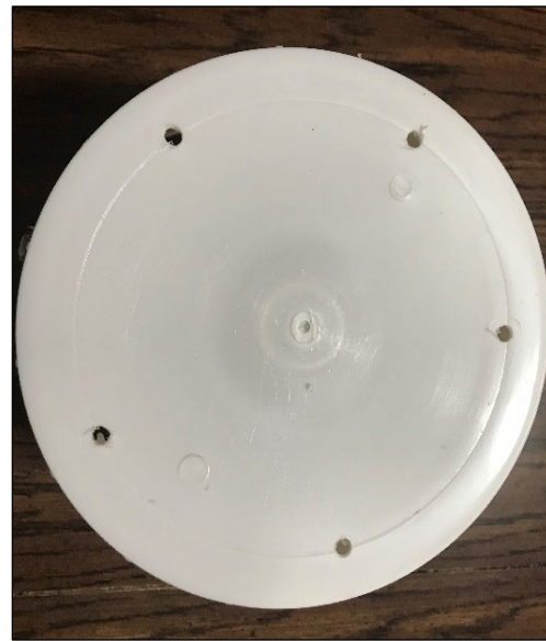
Figure 11 Bucket with five drilled holes
