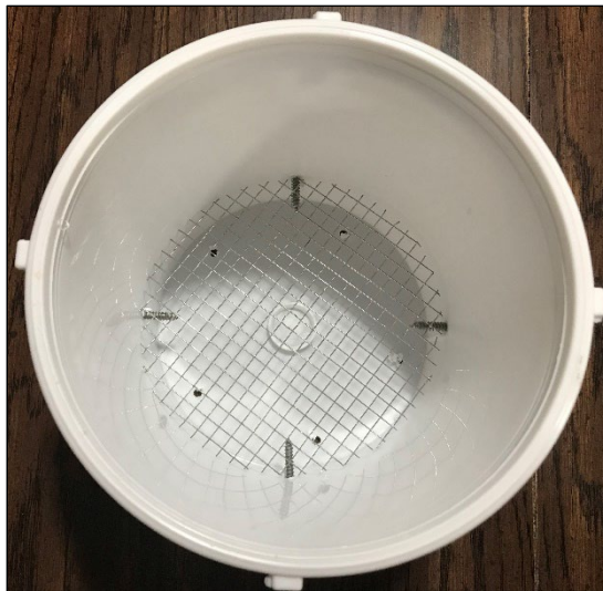
Figure 16 Wire mesh screen placed on machine screws inside bucket trap
