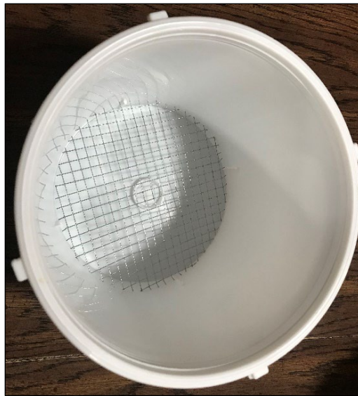
Figure 13 Wire mesh screen in bucket
