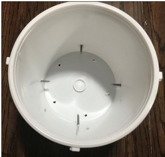
Figure 14 Machine screws placed equal distance from each other around the bucket trap
