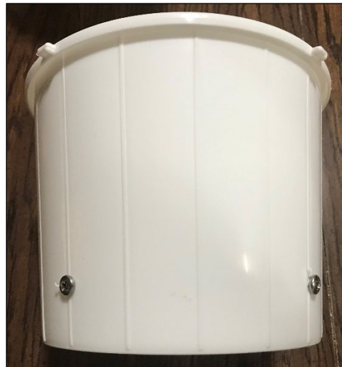
Figure 15 Machine screws shown one inch from the bottom of the bucket trap
